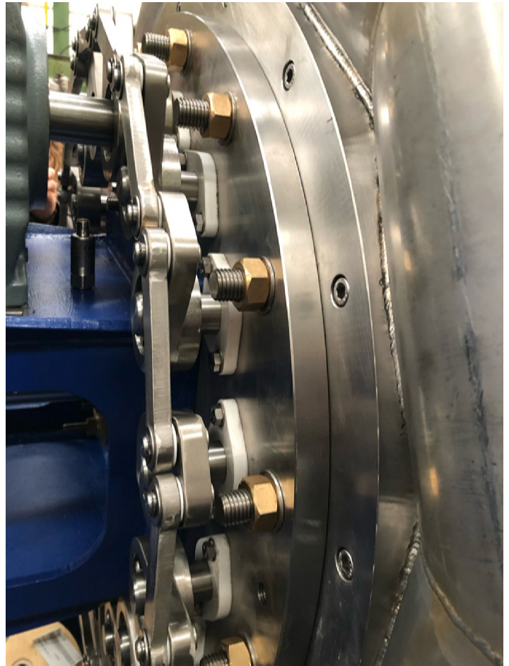
Vesconite Hilube wicket gate bushings are operating successfully at various hydropower plants.
