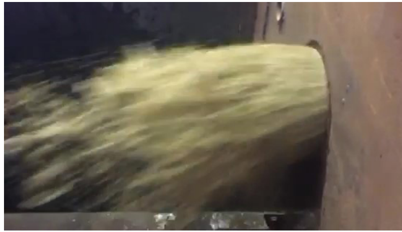
The discharge of a mixture of water and sediments pumped by the slurry pulsejet engine.
