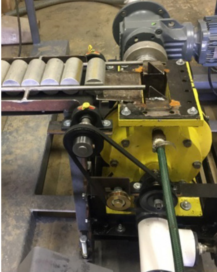
Mazdak's capsule pump launcher being loaded with capsules from a conveyor.
