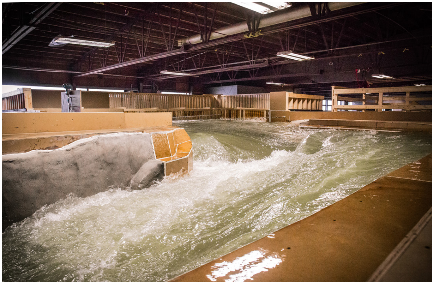
A physical hydraulic model of a spillway located at a hydropower plant in the southeastern United States.
