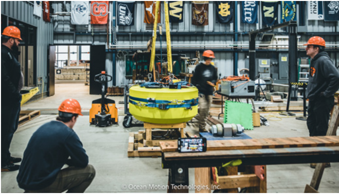
Ocean Motion Technologies personnel prepare the company's wave energy converter for testing at Oregon State University's Hinsdale Wave Research Laboratory.
