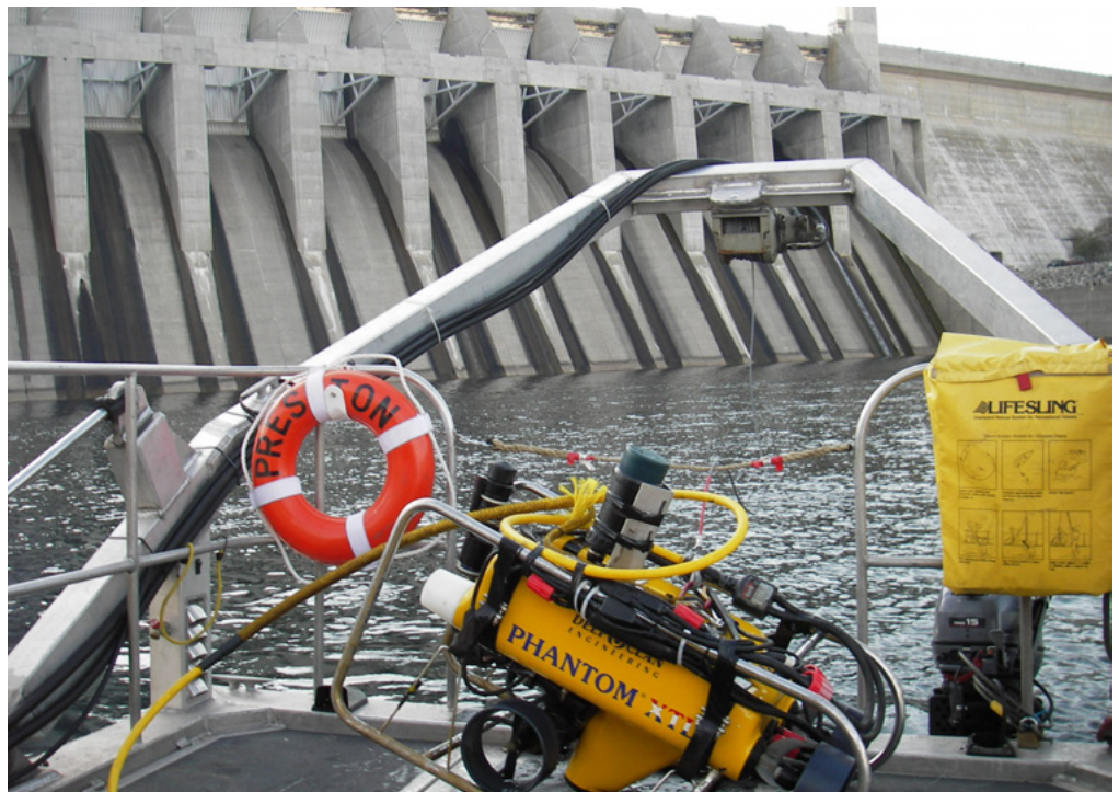
An ROV prepped for deployment from a DEA survey vessel for underwater video inspections of a hydropower dam.
