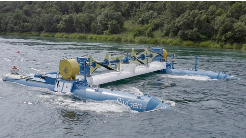
The Village of Igiugig, Alaska, installed its first RivGen hydrokinetic turbine in 2019 as part of a multiyear effort launched in 2018 via a WPTO award.
